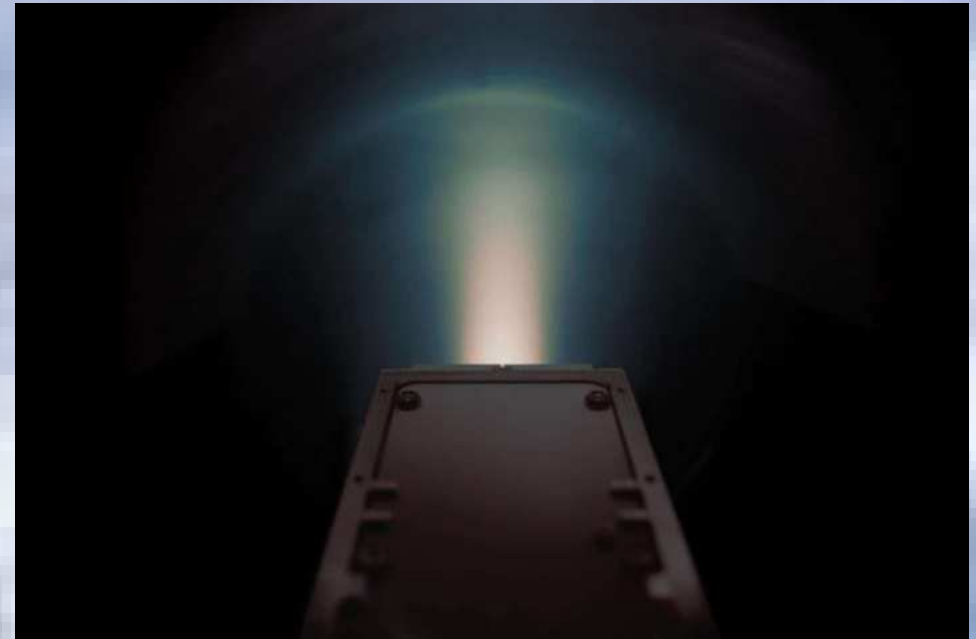
The iodine electric propulsion system firing in a vacuum chamber –M/s.TrustMe
